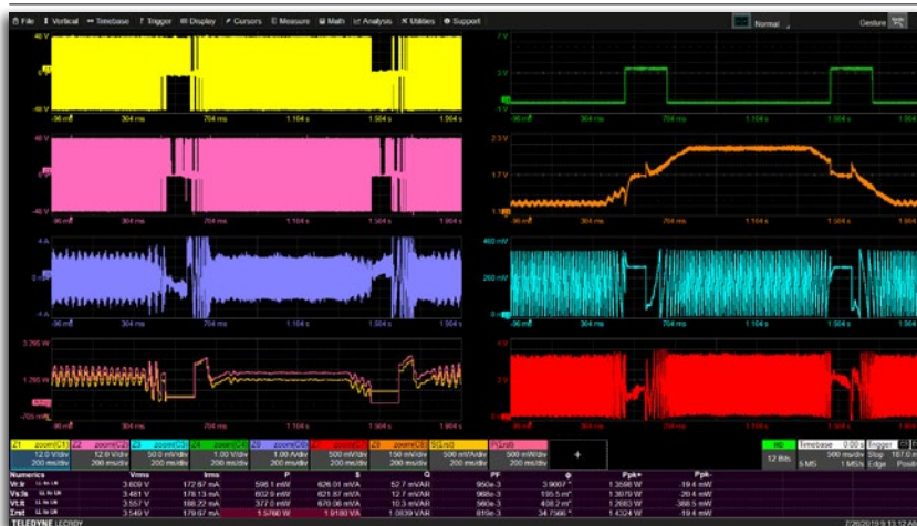
Drive control and feedback signals are compared to drive output voltage and current and calculated power Waveforms to understand whether motor reversal is performing correctly.
