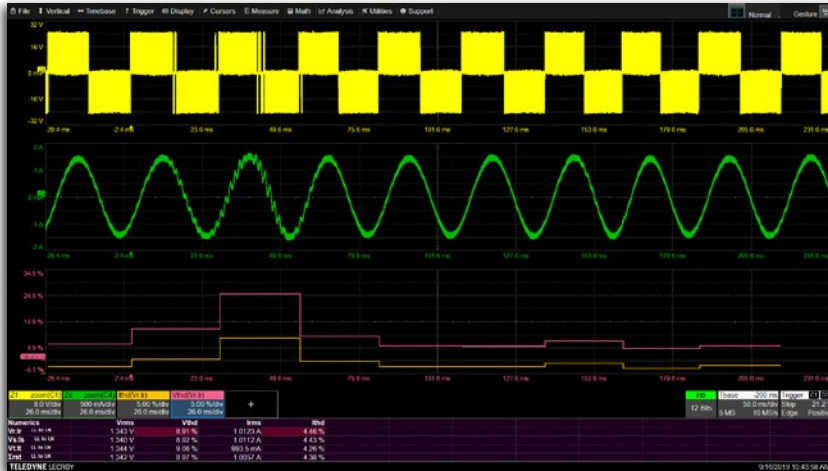
This simplified example shows THD for voltage and current (bottom magenta and orange Waveforms) plotted over time with one THD value per power cycle.
