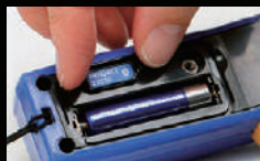
Attach to enable Bluetooth® wireless technology
